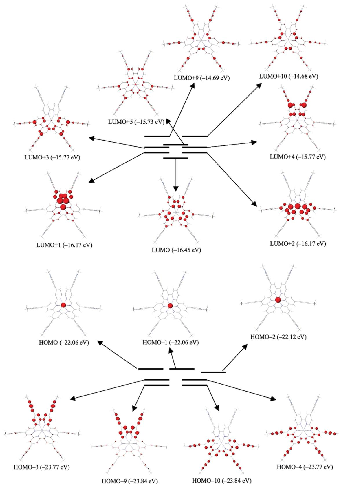
**Figure 5.** The electronic density distribution of the frontier molecular orbitals of the complex cation in salt 1. For the sake of clarity, the electronic density is magnified by a relative ratio of 10, except for the HOMO, HOMO-1, and HOMO-2 orbitals.
