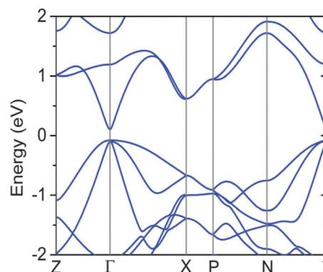
Fig. 1 Band structures of CuInTe<sub>2</sub>.
