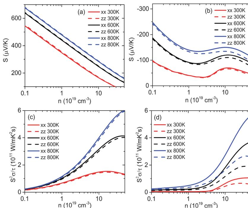
Fig. 5 Anisotropic thermoelectric transport properties of  $\text{CuInTe}_2$  as a function of carrier concentrations at different temperatures: p-type Seebeck coefficients (a), n-type Seebeck coefficients (b), p-type power factors  $S^2\sigma/\tau$  (c), and n-type power factors  $S^2\sigma/\tau$  (d). Here the  $xx$  and  $zz$  directions correspond to the  $a$ -axis and the  $c$ -axis, respectively.
