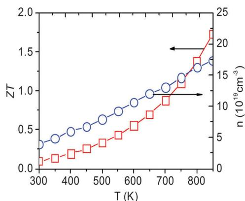
Fig. 7 Optimized figure of merit of p-type  $\text{CuInTe}_2$  and the corresponding carrier concentrations as a function of temperature.
