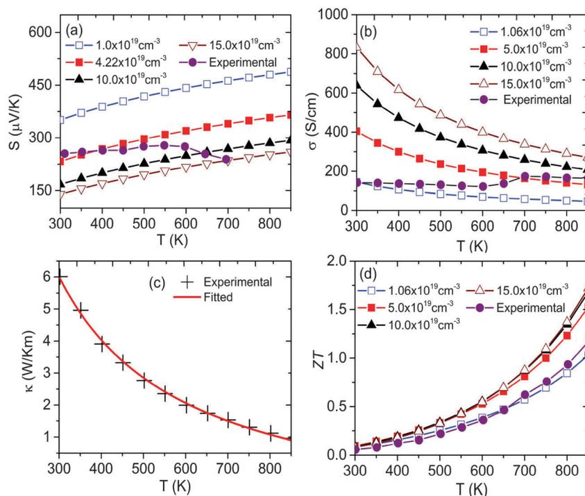
Fig. 6 Seebeck coefficient (a), electrical conductivity (b), phonon thermal conductivity (c) and figure of merit (d) of p-type CuInTe<sub>2</sub> as a function of temperature at different carrier concentrations. The experimental data are plotted for comparison.
