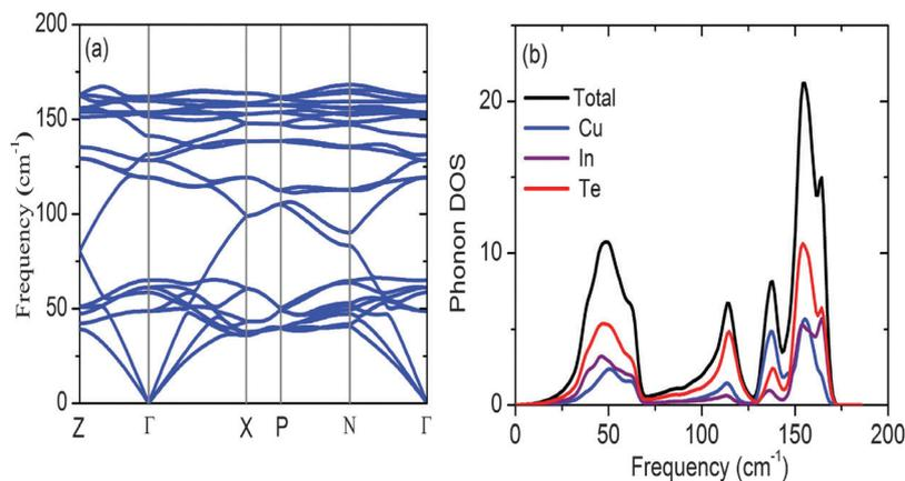
Fig. 4 Phonon dispersion curves (a) and total density of states (b) for  $\text{CuInTe}_2$ . The partial phonon DOS projected onto Cu, In and Te atoms are also shown.
