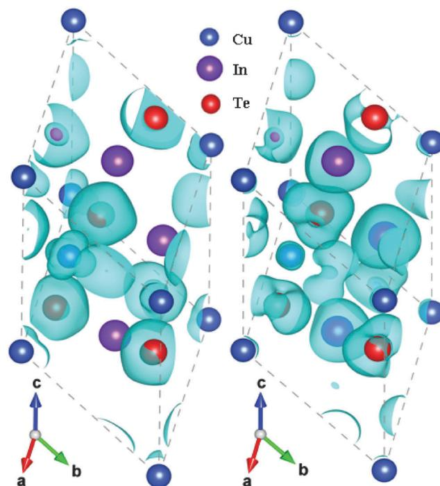
Fig. 3 Partial charge density of CuInTe<sub>2</sub> for the bands near the Fermi level. The left panel represents the upper parts of valence bands within a 2 eV window below the VBM, with an isovalue of 0.0025 e bohr<sup>-3</sup>; the right panel represents the lower parts of conduction bands within a 2 eV window above the CBM, with an isovalue of 0.0035 e bohr<sup>-3</sup>.
